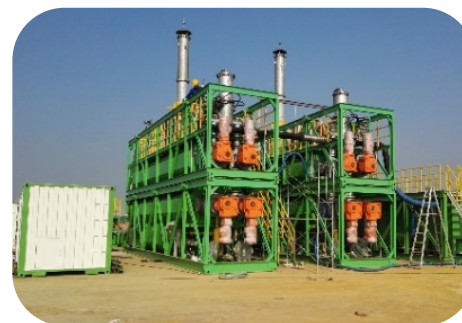
6t/h Soil Thermal Desorption
