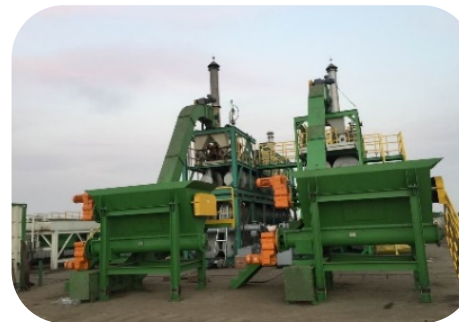
4t/h Oily Soil Thermal Desorption
