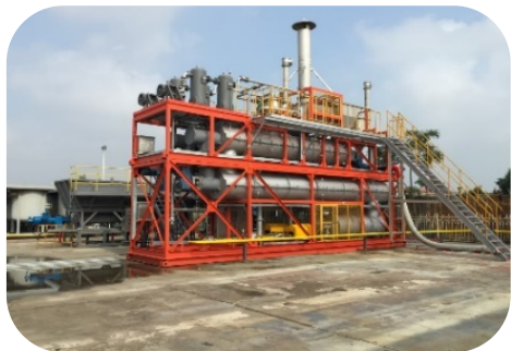
2t/h Oily Sludge Thermal Desorption
