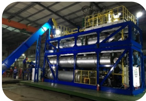
1.5t/h Drilling Cuttings Thermal Desorption
