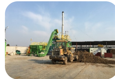
1.5t/h Oily Sludge Thermal Desorption
