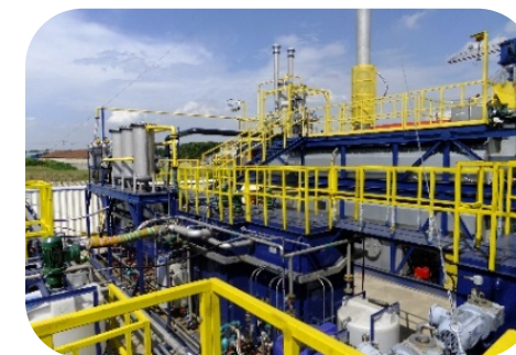
3t/h Dual Plant Thermal Desorption
